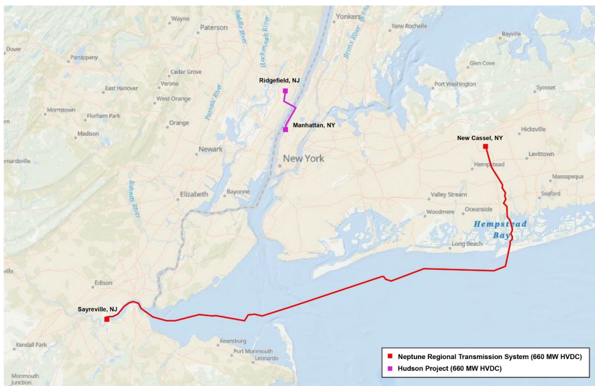
Figure 1-1 Neptune Project and Hudson Project routes
