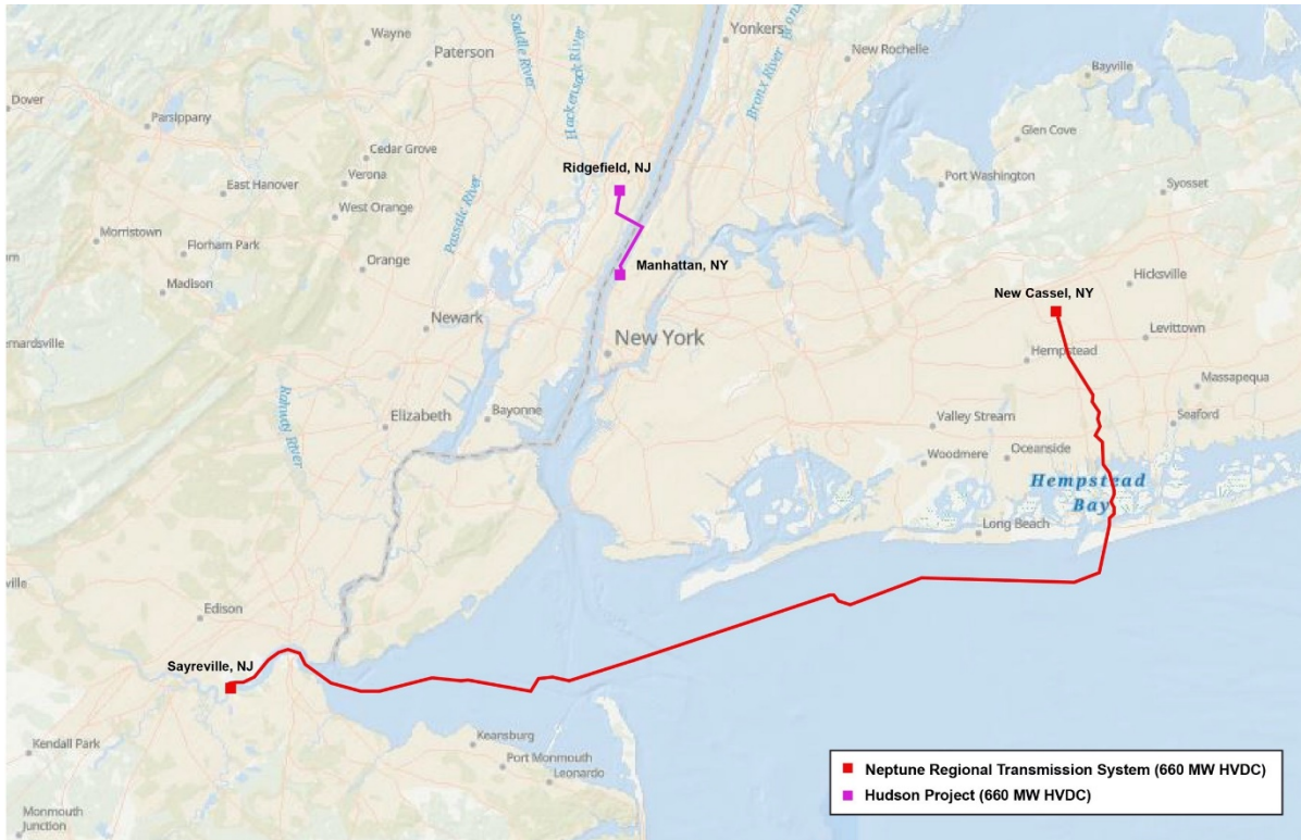
Figure 1-1 Neptune Project and Hudson Project routes
