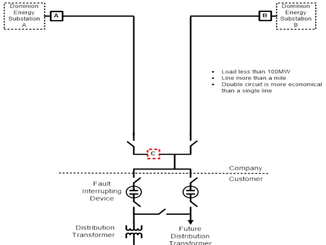
A transmission line tap, as shown in Diagram 4.3.C, can generally be used to interconnect a proposed customer Facility of less than 100 MW and when it is more economical to build double circuit rather than a single line. The customer may reserve property for the DEV-ET owned Interconnection station if one is required.
