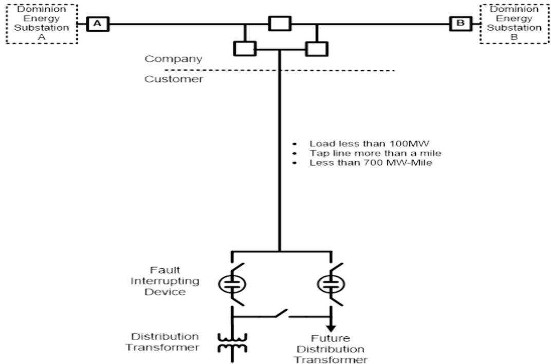
A transmission line tap, as shown in Diagram 4.3.B, can generally be used to interconnect a proposed customer Facility located more than one mile from to the nearest transmission line. A three-breaker or four-breaker ring bus may be required. With this arrangement, the company installs all necessary equipment at the Interconnection substation at or near the transmission line.
