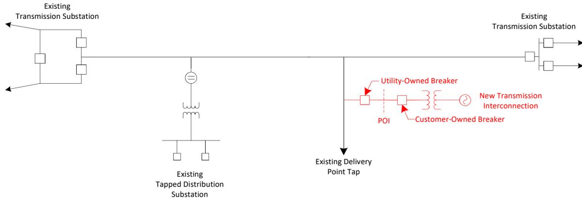
**Figure 3: Typical Tap Line Customer Generation Interconnection Station (Generation Resources  $\leq$  20 MW)**
