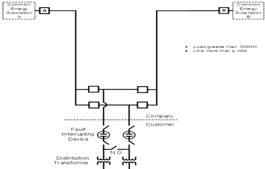
As an alternative to constructing a switching station at the tap point, the transmission line can be cut and looped in and out to a switching station located adjacent to the customer station as shown in Diagram 4.3.E. This arrangement can have its advantages since acquiring land and permitting a new station at the tap point would not be required. The customer should reserve property for construction of the DEV-ET owned Interconnection station.
