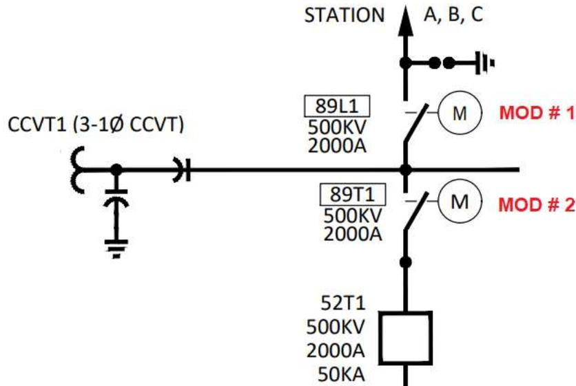
**Figure 2: Example Series Motor Operated Disconnect Configuration**
