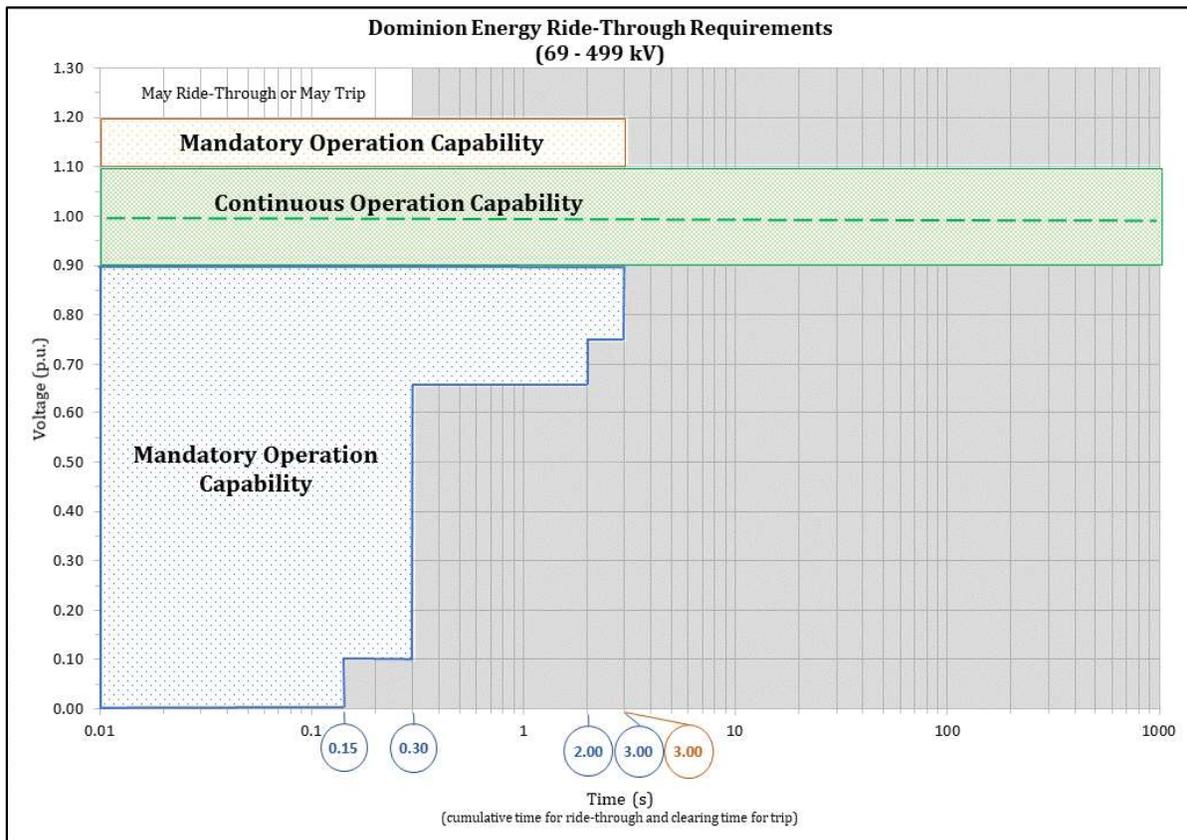
**Figure 1: Dominion Energy Ride-Through Requirements (69 - 499 kV)**
