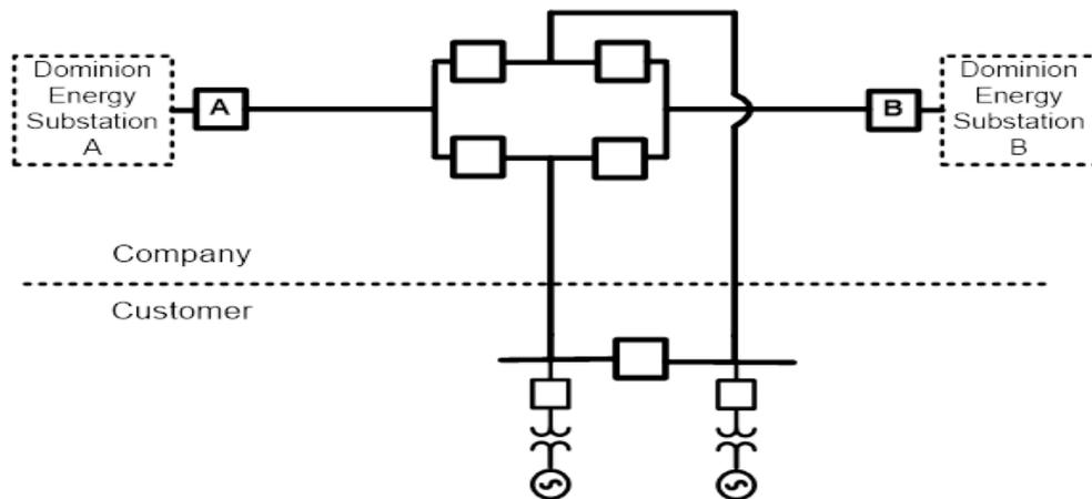
As an alternative to constructing a switching station at the tap point, the transmission line can be cut and looped in and out to a switching station located adjacent to the generating station as shown in Diagram 6.2.B. This arrangement can have its advantages since acquiring land and permitting a new station at the tap point would not be required. The customer should reserve property for construction of the DEV-ET owned Interconnection station.
