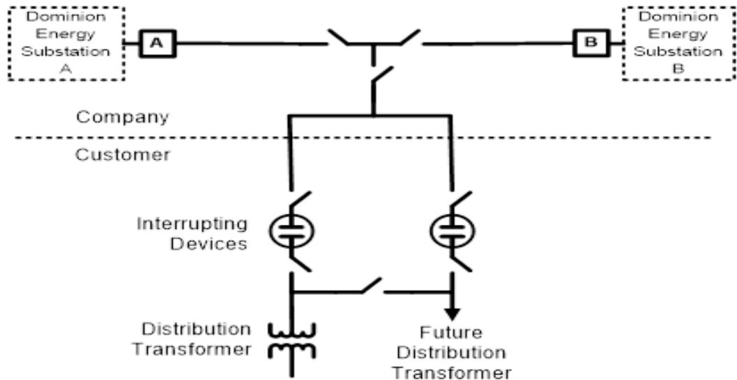
**Diagram 4.4.C.: Allowable sample alternative with fused bypass**
