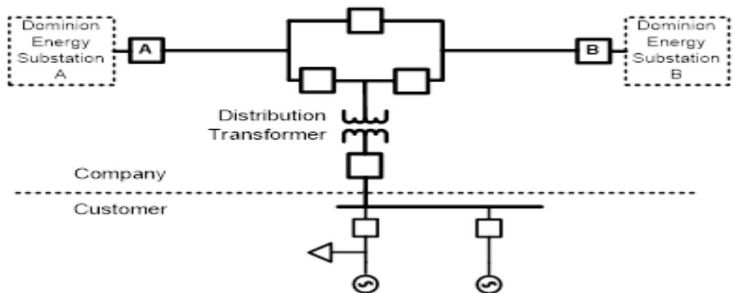
Distribution connected generation resources where the aggregate nameplate rating of all the generating resources (dispersed generation resources) is less than 100MVA can be connected behind a single interrupting device (circuit breaker or circuit switcher).
