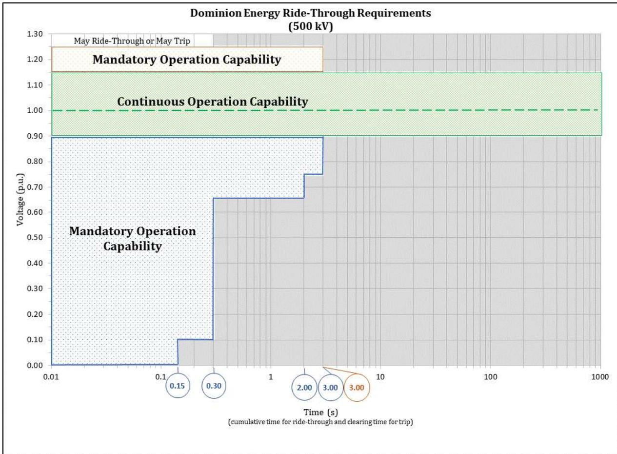
**Figure 2: Dominion Energy Ride-Through Requirements (500 kV)**
