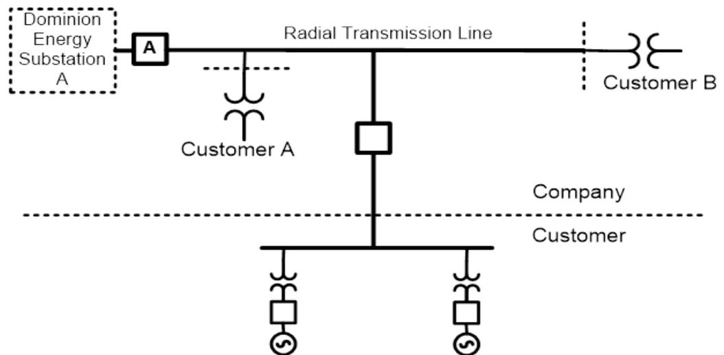
4.2.3.2 A proposed generating Facility may be connected to a transmission tap line portion of a network transmission line, as shown in diagrams 6.3.2.A and 6.3.2.B, subject to Attachment 3 -DEV Generator Interconnection Protection Requirements, Section 3 Interconnection Protection Requirements.
