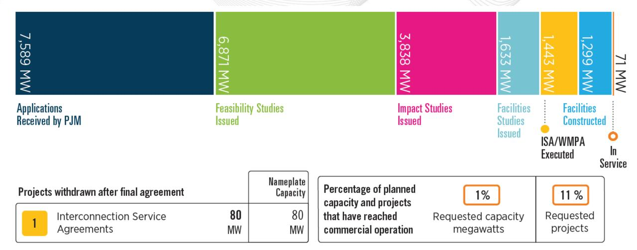
This graphic shows the final state of generation submitted to the PJM queue that completed the study phase as of Dec. 31, 2020, meaning the generation reached in-service operation, began construction, or was suspended or withdrawn. It does not include projects considered active in the queue as of Dec. 31, 2020.
