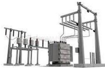
Substation A Limiting Element MVA Rating: 350 MVA Peak Loading in N-1: 125 MVA
