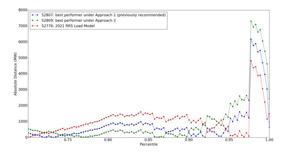
Distances in the extreme upper portion of distribution distort the total distance calculation and therefore, the ranking of load models
