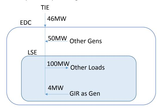
EDC load = 46MW + 50MW + 4MW = 100MW LSE load = 100MW + 0MW = 100MW GIR settled as 3MW load offset, 4MW injection
