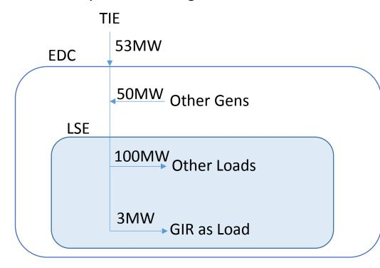
EDC load = 53MW + 50MW = 103MW LSE load = 100MW + 3MW = 103MW GIR dispatched, providing 7MW
