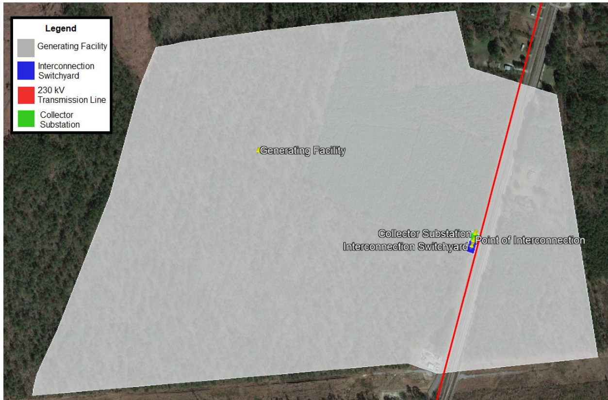
Exhibit XX: Tapping an Existing Transmission Line
