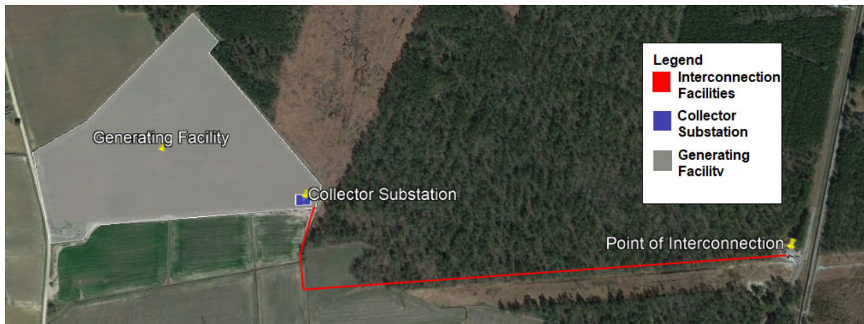
Exhibit xx: Interconnecting into an Existing Substation.
