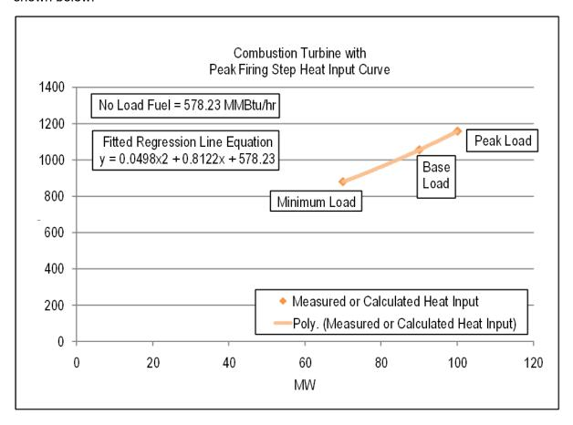
Each diamond in the graph above is a design heat input data point obtained from the original equipment manufacturer or calculated by heat balance. A regression analysis can be performed on the design data to obtain the unit's Heat Input curve as a function of various unit output levels with natural gas as a fuel:
