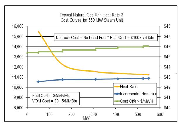
To avoid making adjustments to the No-Load Cost, first calculate the unit's Incremental Cost (\$/MWh) at various outputs using the derivative of the Heat Input Curve:
