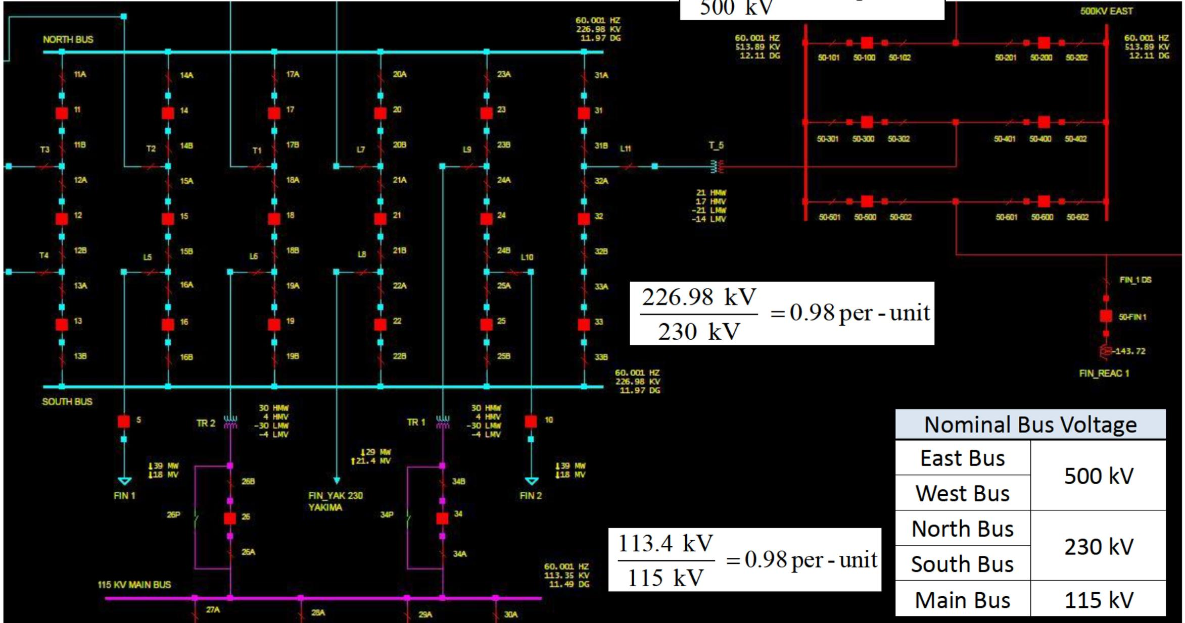
$$\frac{226.98 \text{ kV}}{230 \text{ kV}} = 0.98 \text{ per - unit}$$
