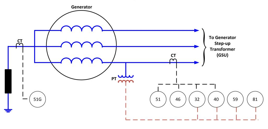
51 – Back-up Overcurrent59 – Over-excitation46 – Negative Sequence81 – Under-frequency32 – Reverse Power (Anit-motoring)51G- Neutral Over-current40 – Loss of Field51G- Neutral Over-current
