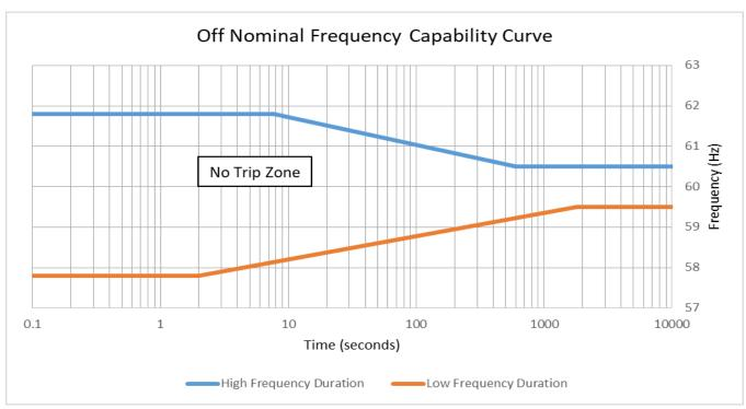
Figure 8: NERC Standard PRC-024 Frequency Ride-Through Capability Curve
