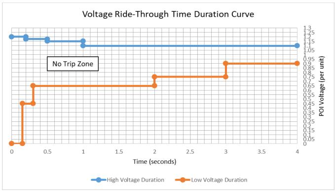
Figure 7: NERC Standard PRC-024 Voltage Ride-Through Duration Curve
