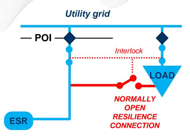
Interlock among switches allows closed resilience connection only when disconnected from grid on both sides.
