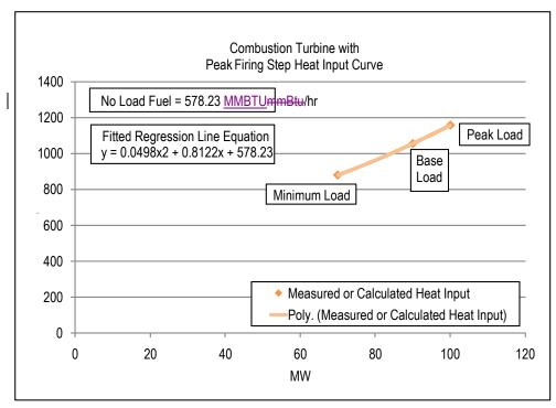
Each diamond in the graph above is a design heat input data point obtained from the original equipment manufacturer or calculated by heat balance. A regression analysis was performed on the design data to obtain the unit's Heat Input curve as a function of <u>unit's o</u>Output with natural gas as a fuel:
