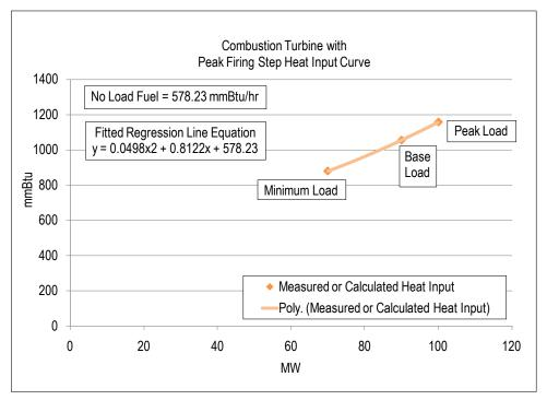
Each diamond in the graph above is a design heat input data point obtained from the original equipment manufacturer or calculated by heat balance. A regression analysis can be performed on the design data to obtain the unit's Heat Input curve as a function of <a href="mailto:various">various</a> <a href="mailto:unit o\text{-}unit o\text
