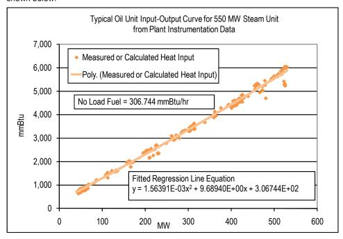
Each diamond in the graph above indicates one hourly heat input data point calculated from plant instrumentation during operations. A regression analysis was performed on the data collected to obtain the unit's Heat Input curve as a function of unit's oQutput with oil as a fuel:
